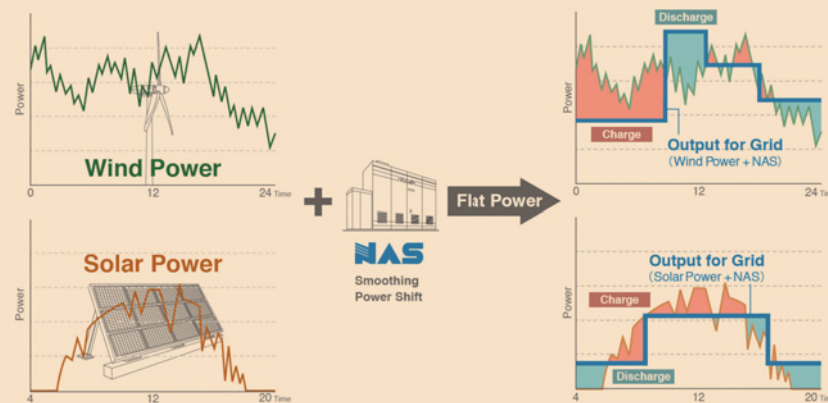
Box figure A1.6.2.1 Use of NaS batteries for peak shaving
